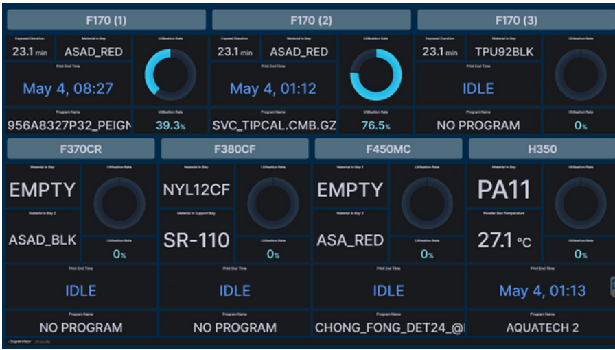
An overview of seven 3D industrial printers in a dashboard for operators.
